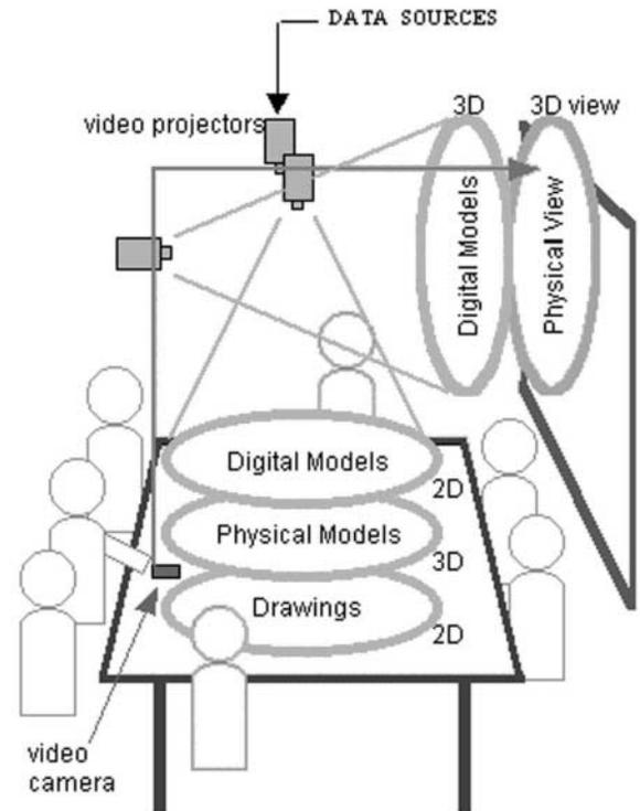
**Figure 2.** Luminous Planning Table integrates digital and physical mediums.
